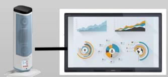
Some newer interactive screens use a HDMI connector. This also carries the audio to the screen and isolates the headphone socket on the laptop. The screen often will give you a headphone socket or audio output (seen to the left). Simply use an audio lead from the screen and connect to the JUNO audio input.
